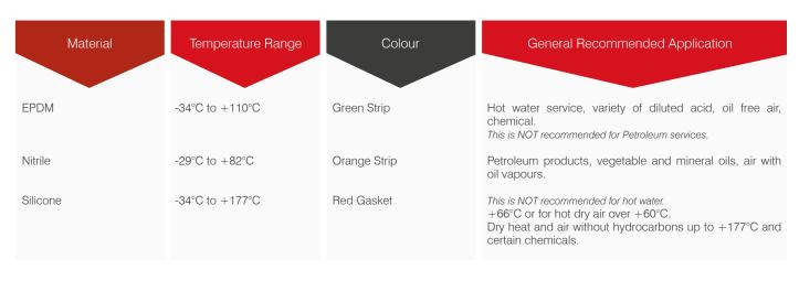
SHIELD Grooved Coupling EPDM Gaskets must be lubricated on the lips and outside back prior to assembly using silicon based non-petroleum lubricant. For more details about lubricant for other types of gasket, please contact us.
